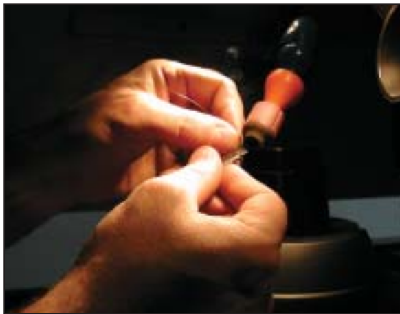
Filler wire being applied during laser weld process.
